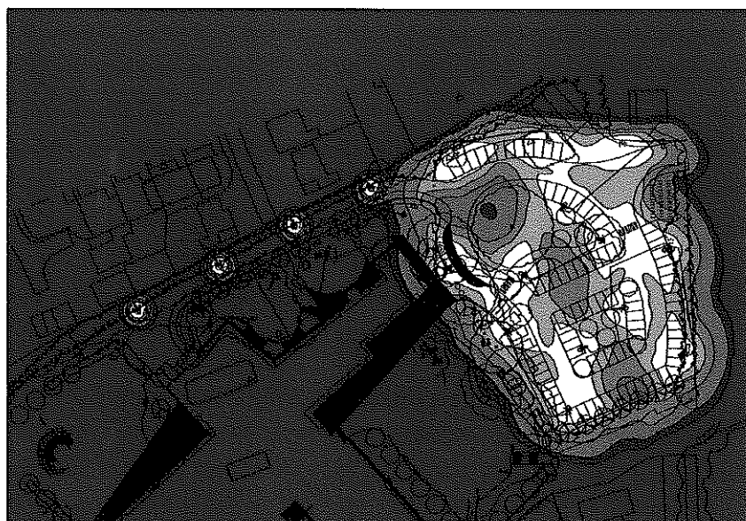
Figure 2: Light spill of proposed scheme following the replacement of service road column lighting with bollard lighting.
